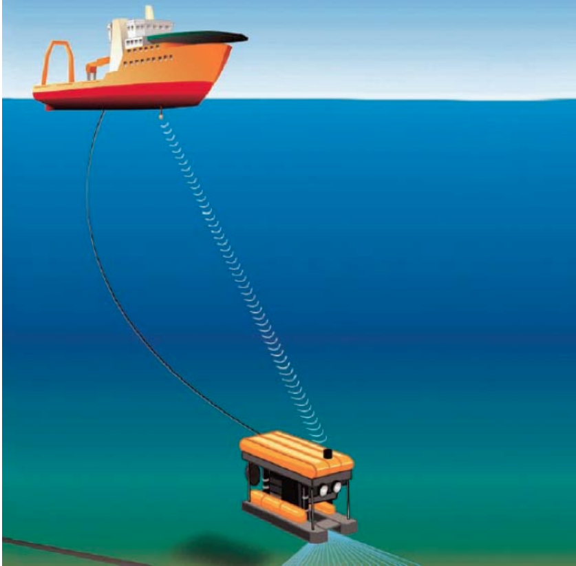
Figure 2.8: Ultra Short Baseline acoustic positioning system, courtesy of Kongsberg Maritime
