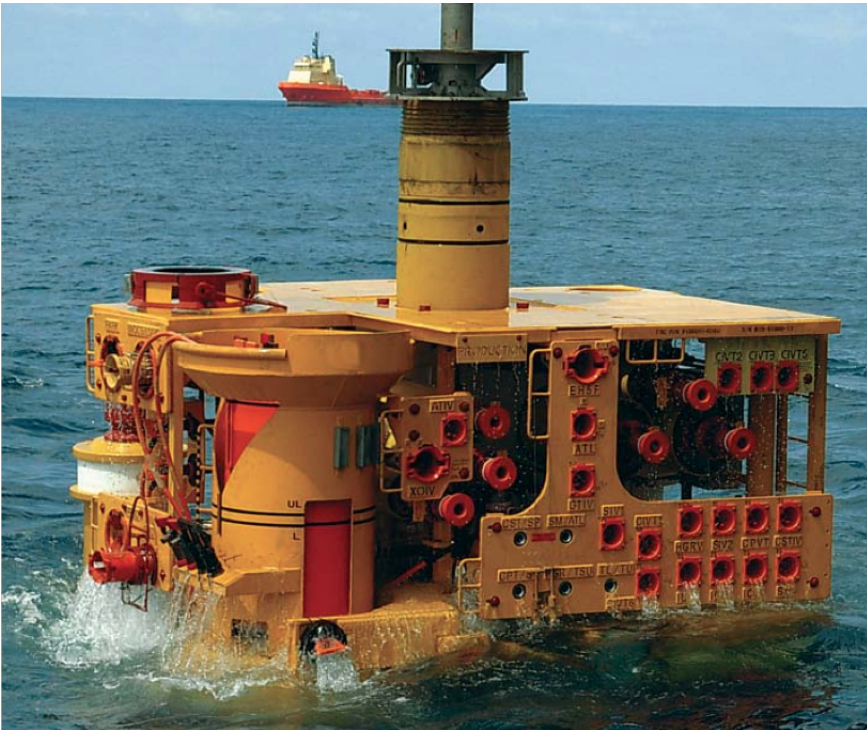
Figure 2.2: Photo of Xmas tree during installation, courtesy of FMC Technologies
