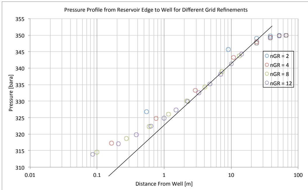
Figure 2.19 – Pressure profiles for different grid refinements around the lateral blocks. A hydrostatic correction has been made. The pressure in the center block is not included. The distance is measured from the center of the well.
