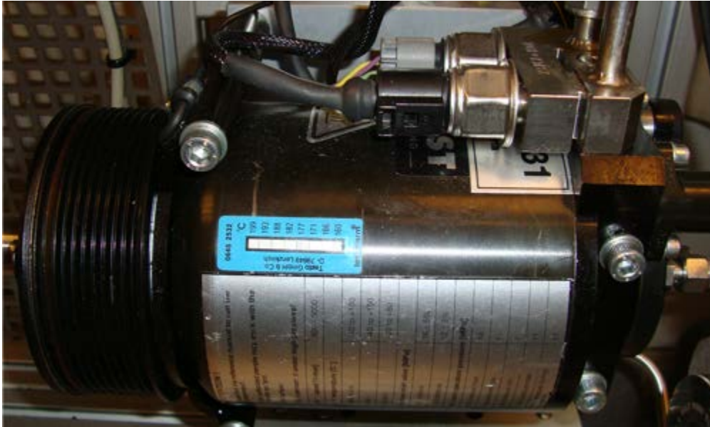
Figure 21 The CO 2 compressor C99-5 with variable displacement
