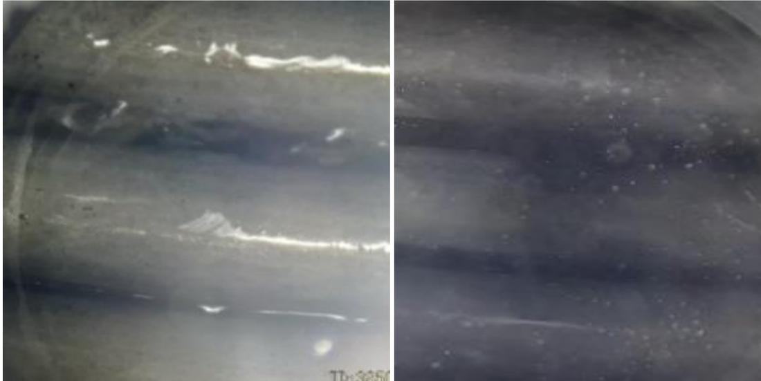
*Figure 5-14 – left: Falling film flow and Right: Intermittent flow. Propane at 4.5 bar from observations at the Lab set up in SJTU.*
