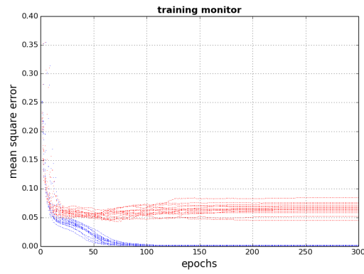
(b) Example of over-training. The errors of the training set go down while the errors of the validation set go up or stay constant.
