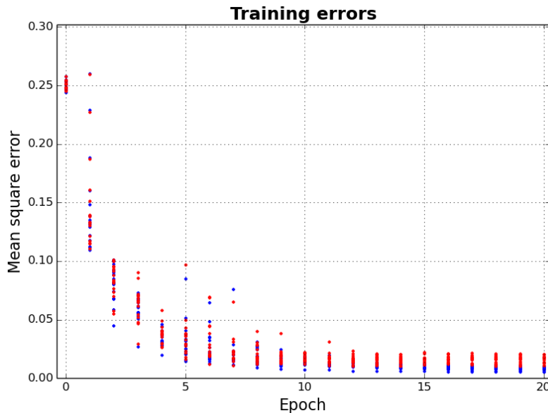
Figure 4.14: The training errors are shown for the final training data and for a random subset of ANNs. Red markers show the validation errors and the blue points represent the training errors. Ten epochs seem to be optimal for training.
