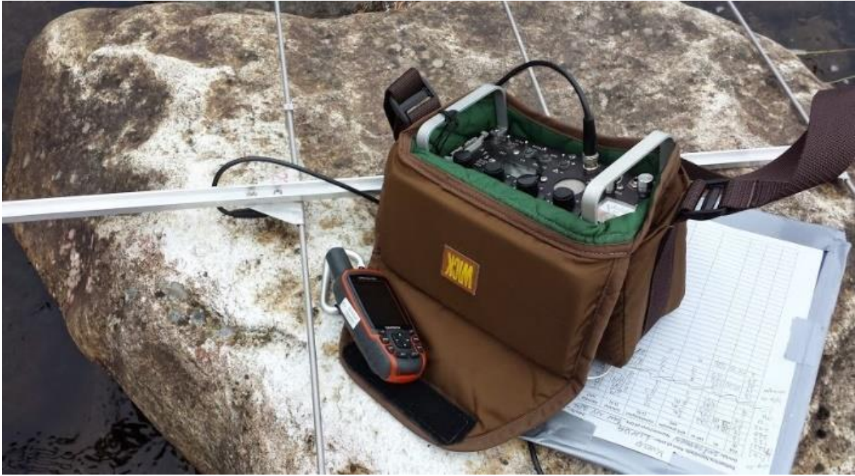
Picture 1 Receiver, antenna, GPS and habitat form used for radio tracking
