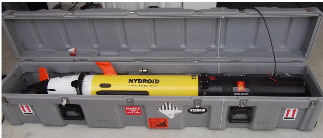
(a) REMUS 100 AUV in its transport box
