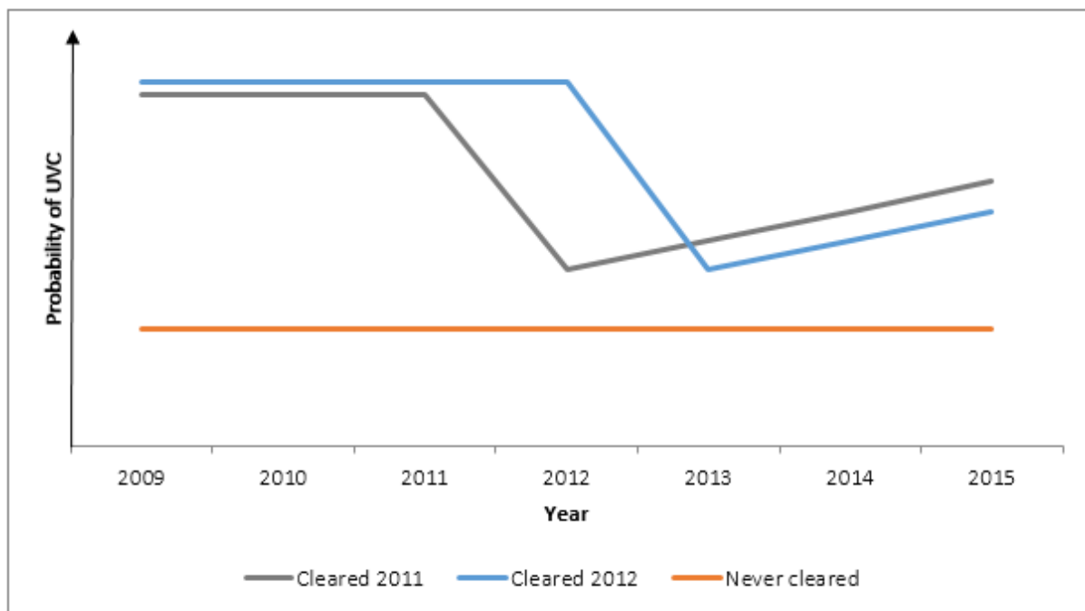
Figure 1. A conceptual illustration of the predicted responses in probability of UVC following clearing of roadside vegetation in Nord-Trøndelag County in 2011 or 2012, given that density and environmental effects are constant.
