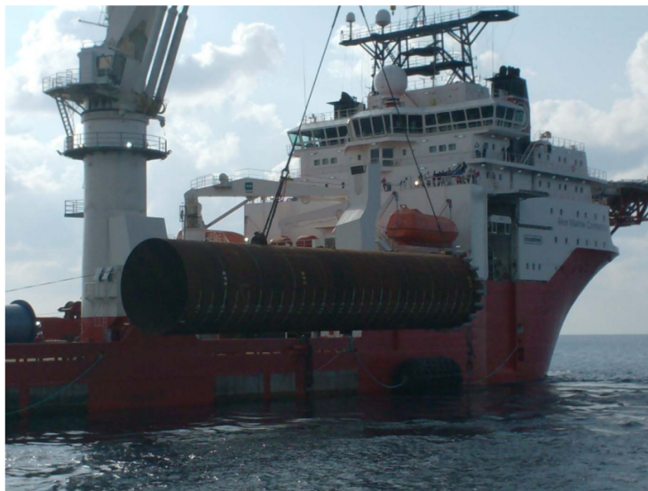
Figure 2.1: Lifting of Suction Pile (Parimi and Qian; 2008)
