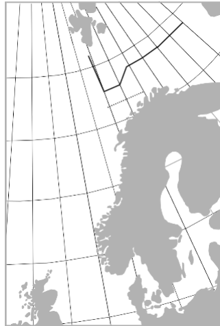
Figure 3.2: Limit for collision with icebergs with a probability of exceedance of 10^{-2} (solid line) and 10^{-4} (dotted line) (Standards Norway, 2007).
