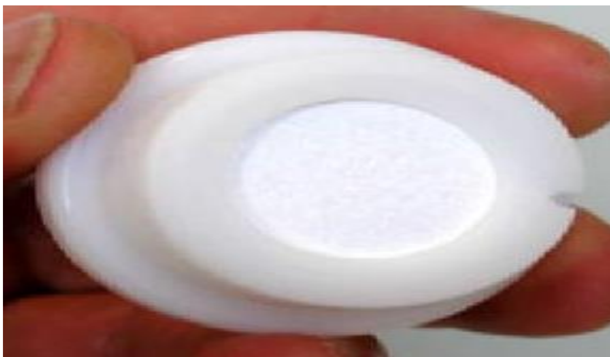
Figure 4.7 A DGT unit sampler taken out of seawater sample and ready for the separation of the three layers.
