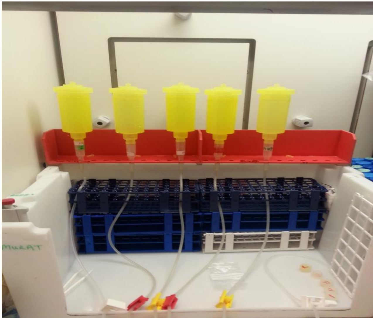
Figure 4.6 The set up for Chelex-100 pre-concentration columns for iron and other trace metals.
