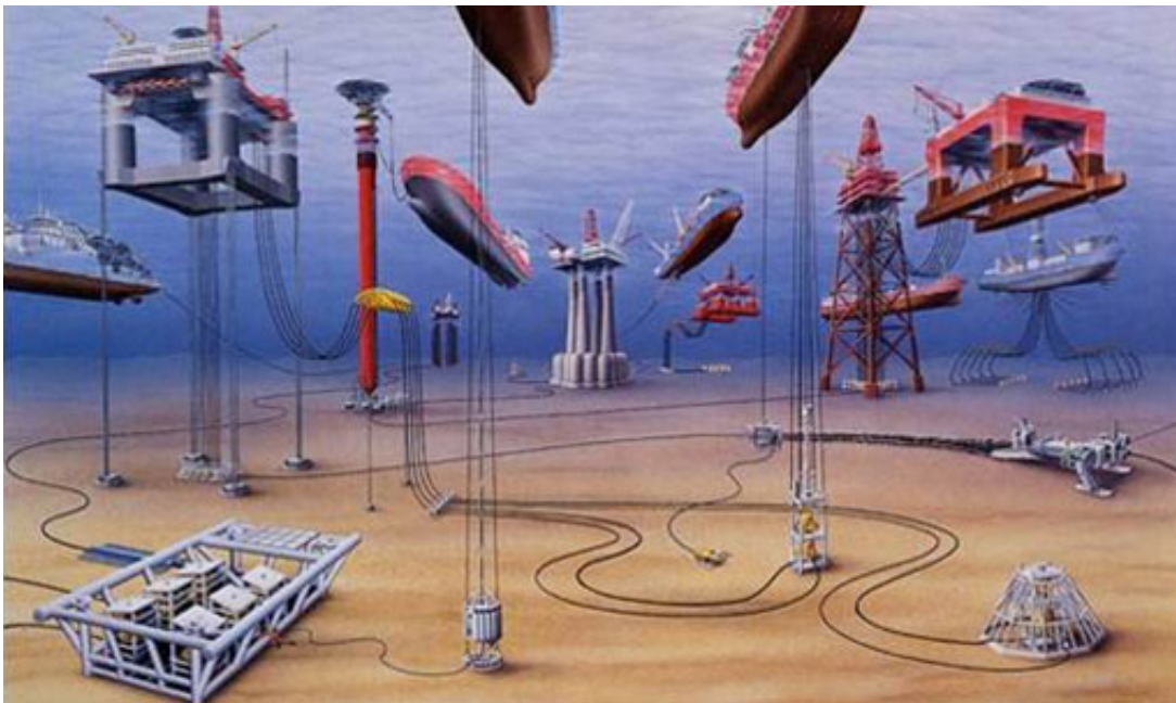
Figure 1.1: Flexible riser system
