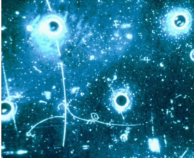
Figure 3.7: The first example of a single-electron neutral current. An incoming antineutrino knocks an electron towards the left, creating a characteristic electronic shower with electron-positron pairs. Credit: Gargamelle/CERN.
