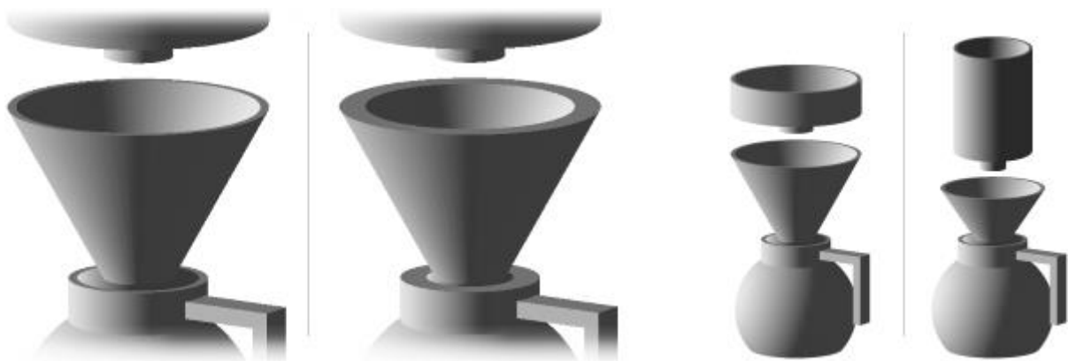
Figure 32: Form variation in AML – changing dimensions (thickness, size)
