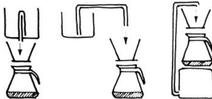
Figure 7: Quantified structure of a coffee maker (adapted from Tjalve, 2003)
