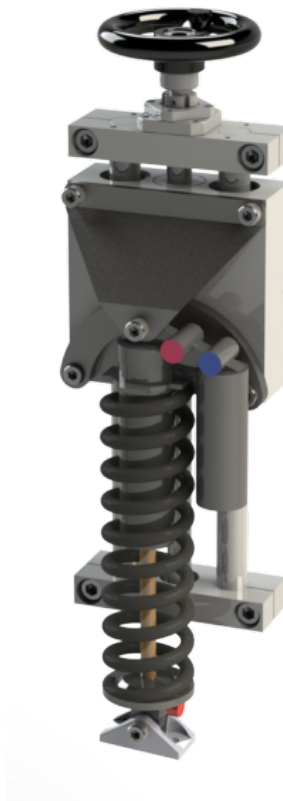
Figure 3.2: Manual actuator combined with a shock absorber to exert normal force on the test ski.
