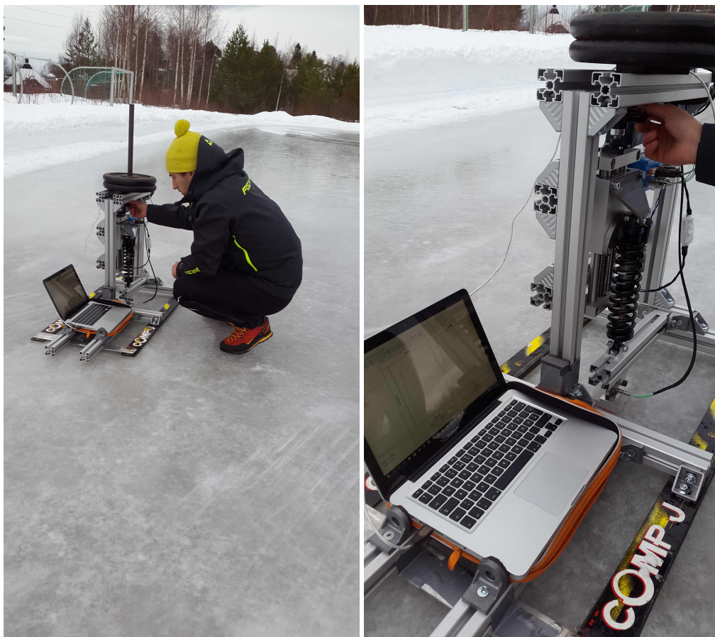
Figure 4.3: Friction meter in action on ice.
