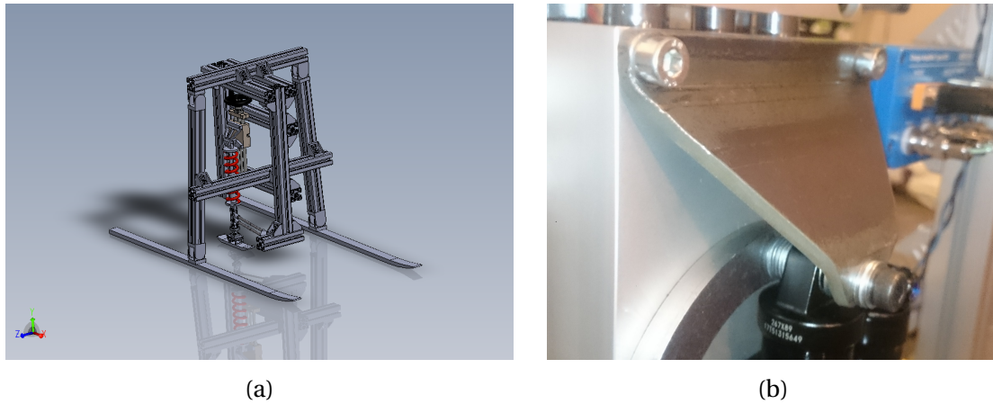
Figure 3.11: a) Tribometer with an early sled design. b) Angled bracket for the transition between the manual actuator and the shock absorber.
