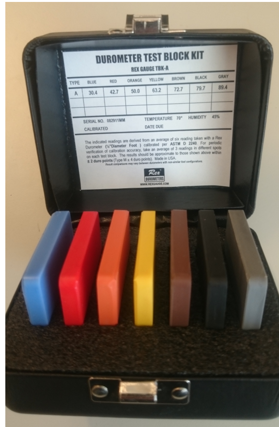
Figure 4.1: Rex Gauge durometer test block kit. Used for friction testing on ice. The dimensions of the rubber blocks are 51mm x 51mm x 7mm.
