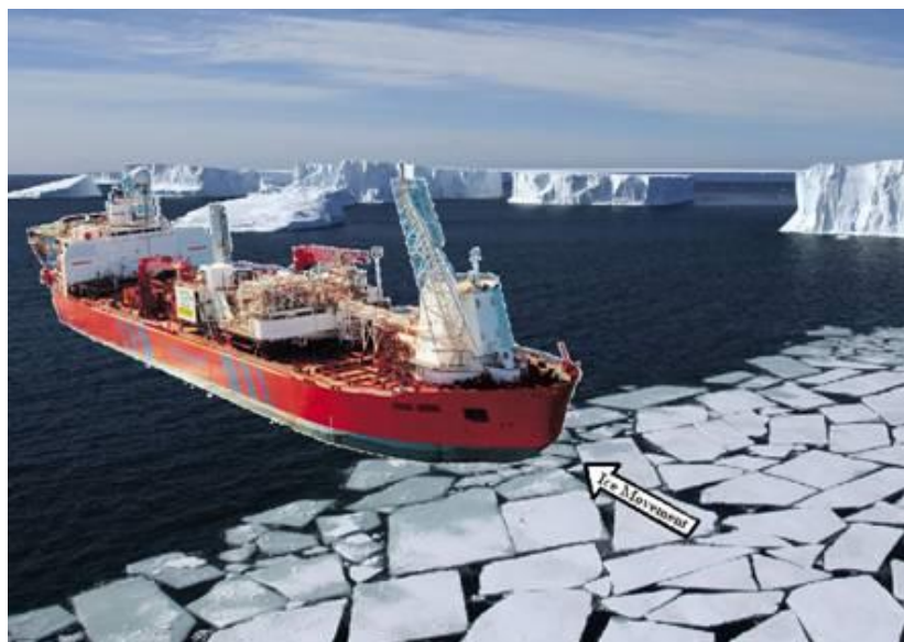
Figure 3-1: Ice vaning: Ice drifts and ship direction [12]
