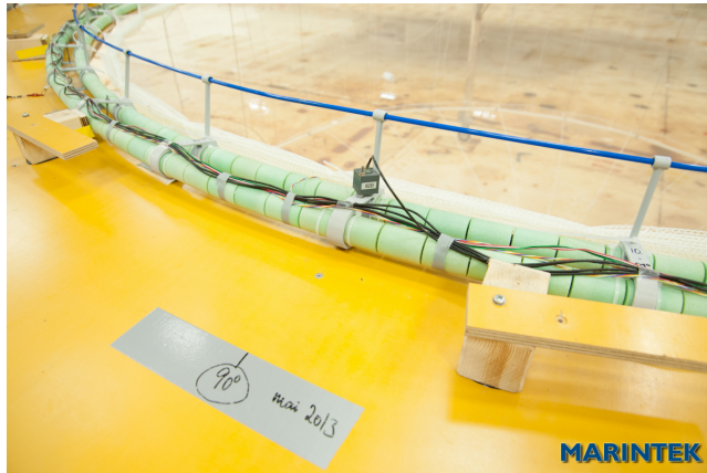
Figure 3.1: Model of a fish farm floater collar consisting of two torus (Nygaard 2013)
