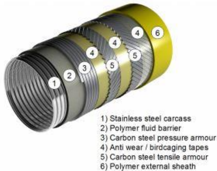
Figure 1 Flexible pipe components[5]
