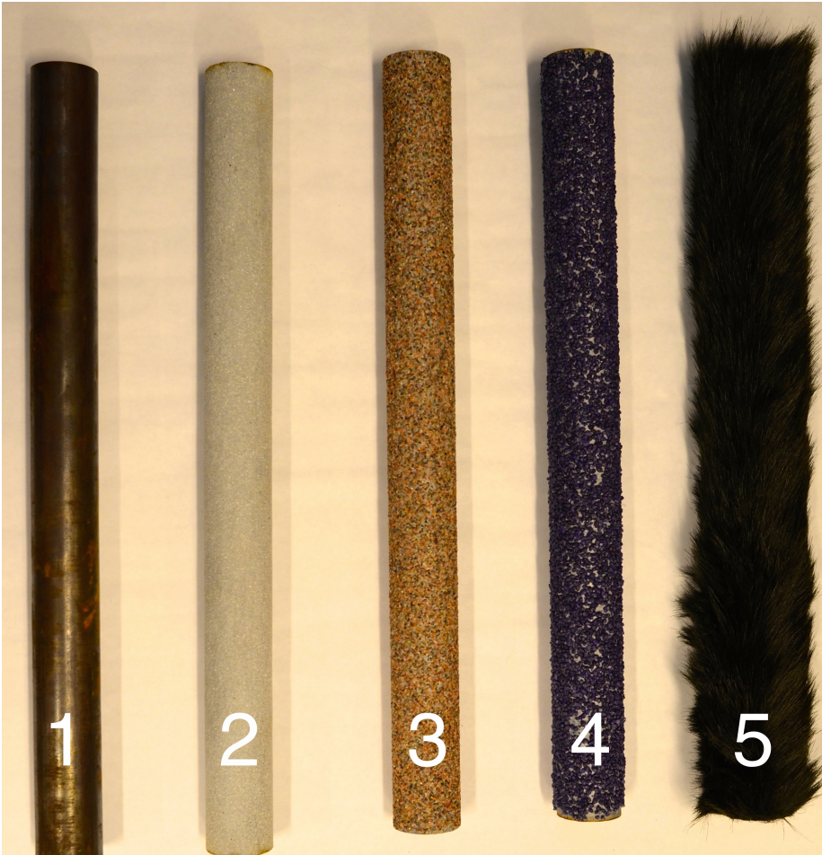
Figure 3.11: The five cylinder models used in the experiment
