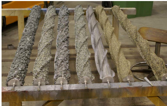
Figure 3.8: Simulation of hard marine fouling on marine risers, from Baarholm (2007)
