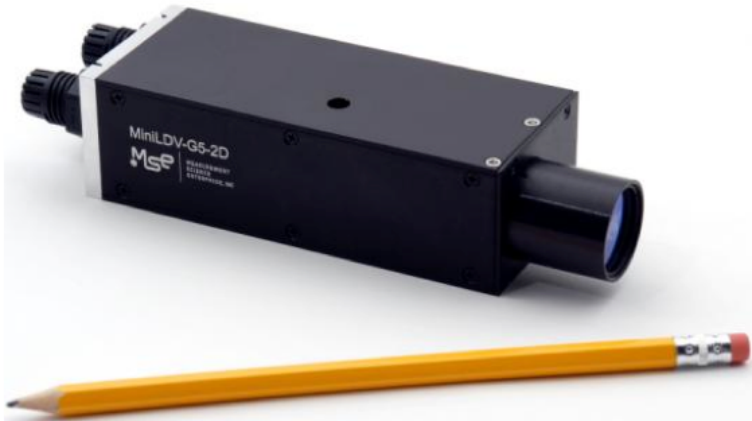
Figure 3.6: 2D miniLDV. From Measurement Science Enterprise Inc. (nd)
