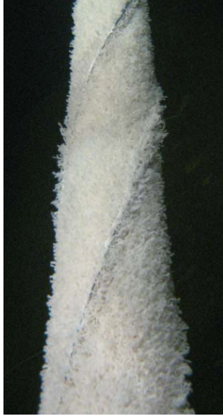
Figure 3.7: Simulation of soft marine fouling on marine risers, from Baarholm and Skaugset (2008)
