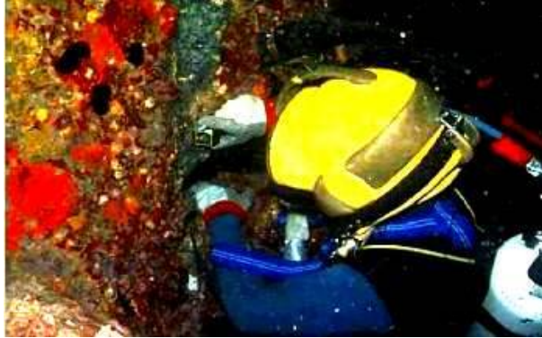
Figure 1.4: Diver performing non-destructive testing [5]
