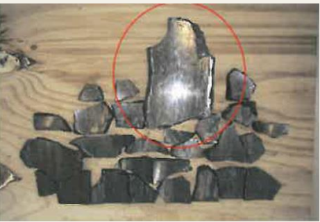
Figure 3: Broken cylinder liner
