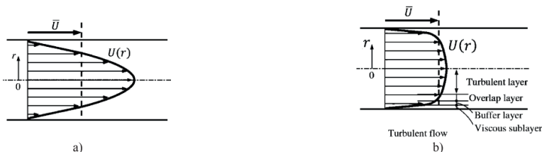
Fig. 1. Fully developed velocity profile in pipes a) Laminar flow b) Turbulent flow. Adapted from Çengel and Cimbala (2010)
