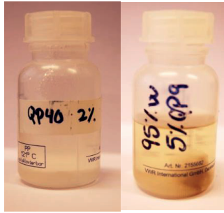
Fig. 3-3 Liquid solutions with 2% QP40, 5% QP09L after some months.
