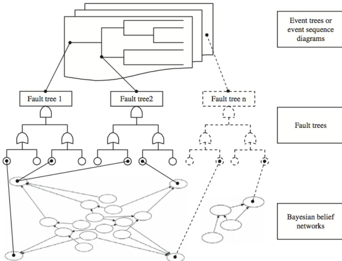
Figure 3.6: The HCL framework. Source: Røed et al. (2009)
