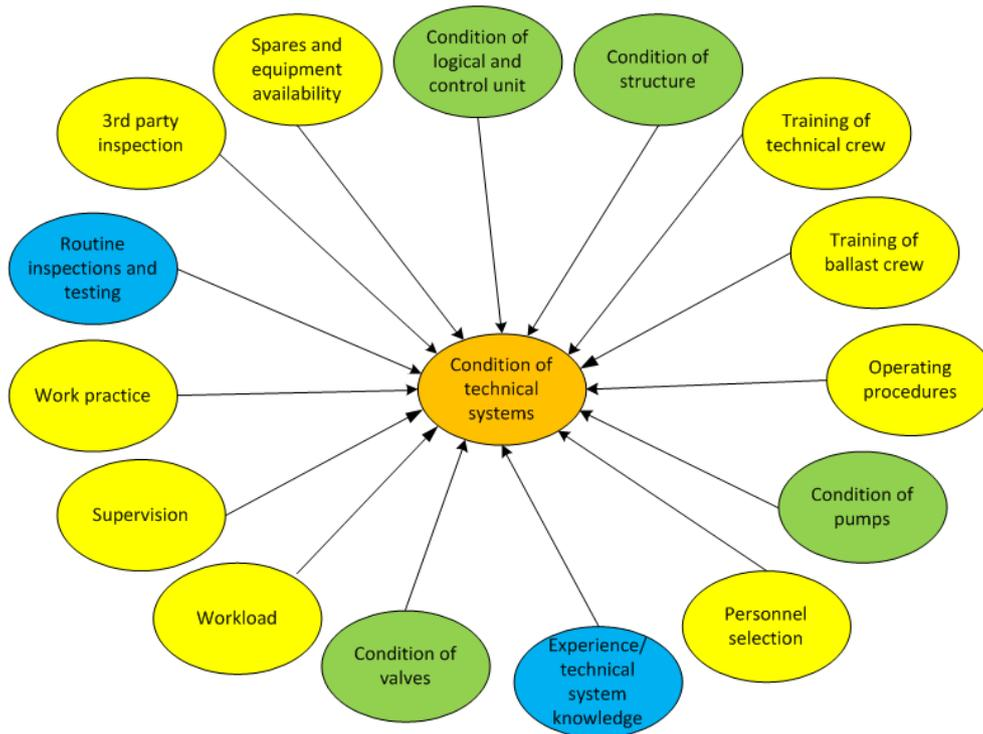
Figure 6.3: RIFs affecting the condition of technical system
