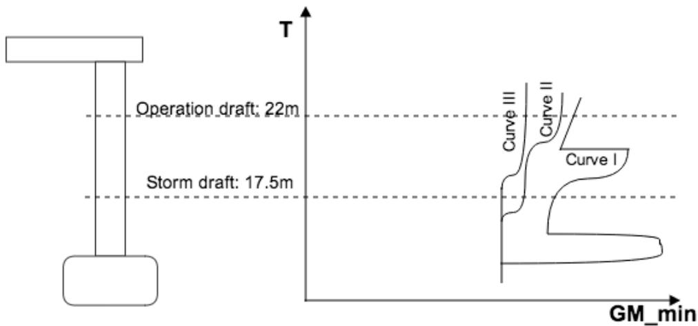
Figure 2.2: Deballasting curve from operation to storm draft. Source: partly based on Sillerud (2013b)
