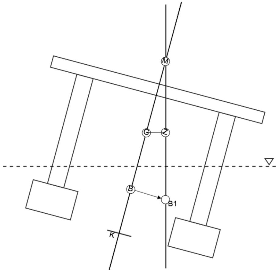
Figure 2.1: Important positions and centers in stability. Source: based on Hancox (1996)
