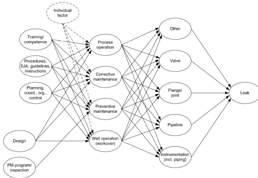
Figure 3.7: ORIM causal network model for leak frequency. Source: Øien (2001a)
