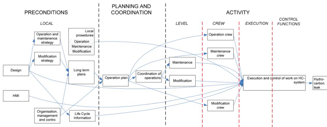
Figure 4.4: Factor model of RIFs influencing the risk of hydrocarbon leaks. Source: Haugen et al. (2012)
