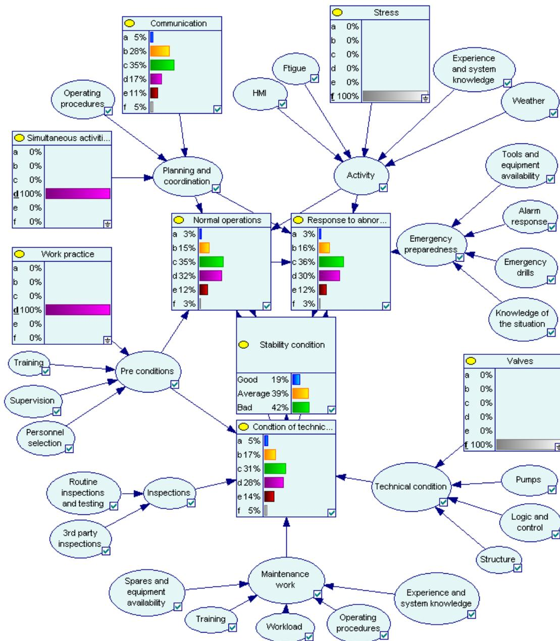
Figure 6.10: Screenshot from GeNIe illustrating the analysis when evidence is provided
