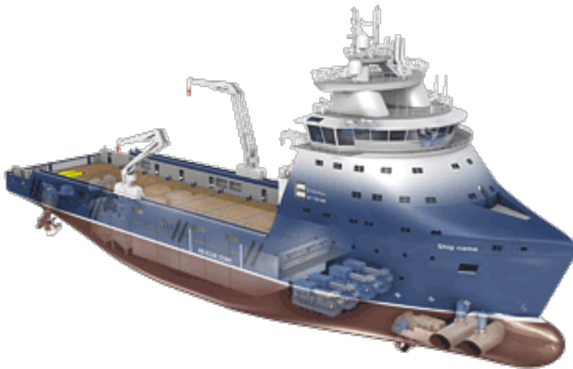
Figure 2-6 Platform Supply Vessel (11)
