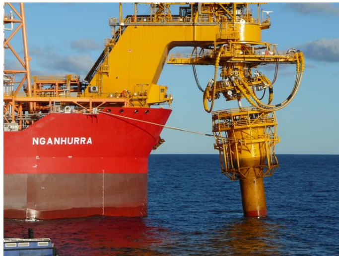
Figure 2.3: Disconnectable turret ( Source: Navicom Dynamics )
