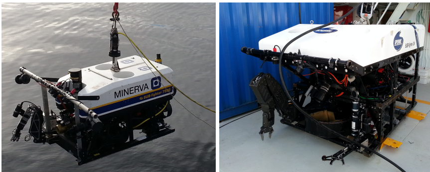
(a) The ROV Minerva being launched.
