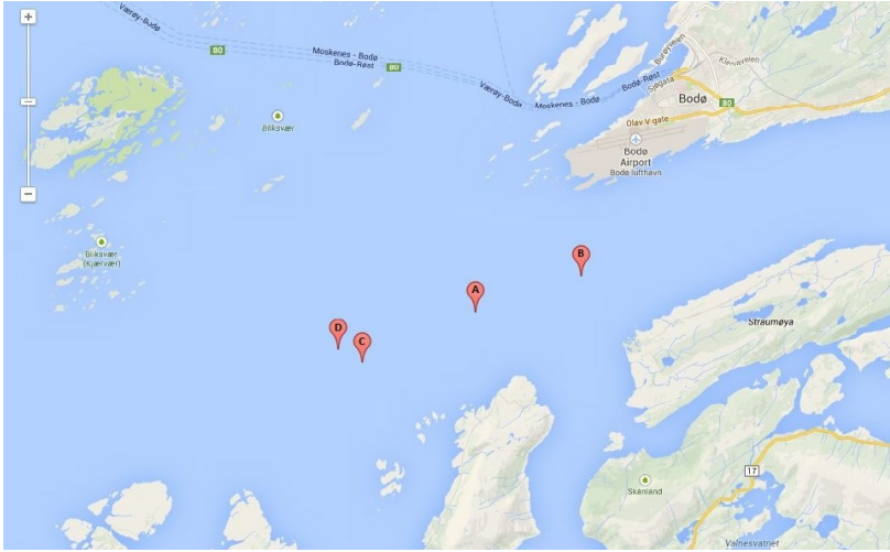
Figure 5.1: MF Landegode's position 30/08/2013. Mark A and B is the position of the port and starboard turning circle, respectively. Mark C and D is the position of the 20/20 and 10/10 zig-zag manoeuvre to port, respectively.
