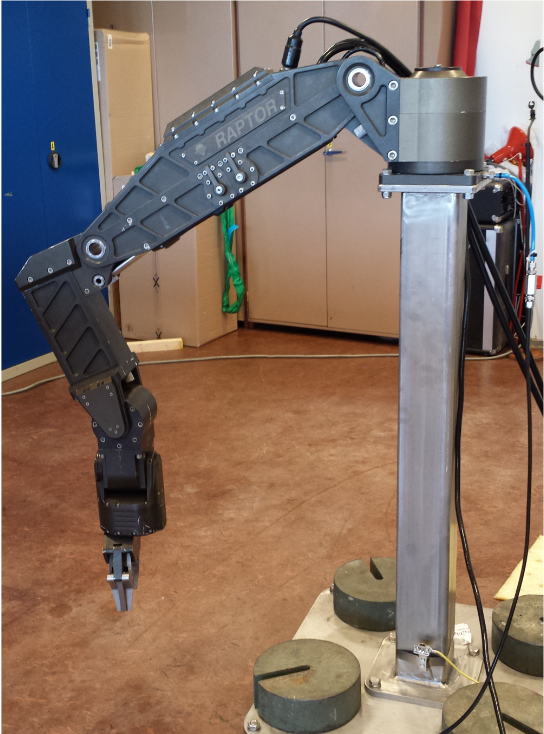
Figure 5.13: The manipulator mounted on the support structure
