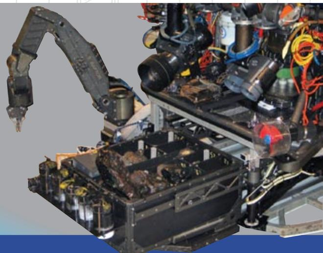
Raptor's close-coupled wrist with 200 degrees of pitch and yaw motion provides high dexterity where its needed most. A high efficiency piston motor delivers "smooth" wrist roll torque, even at fractional RPM. Kraft's unique method of controlling the gripper allows the operator to proportionally vary the rate of jaw closure, and the amount of grip force.
