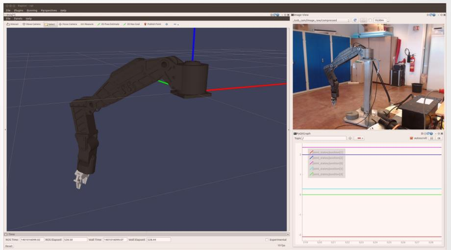
By doing this during operation a real time visualization of the arm is visible at all times. If visual sources such as cameras is unavailable, the operator still has the visualization for support during operations.
