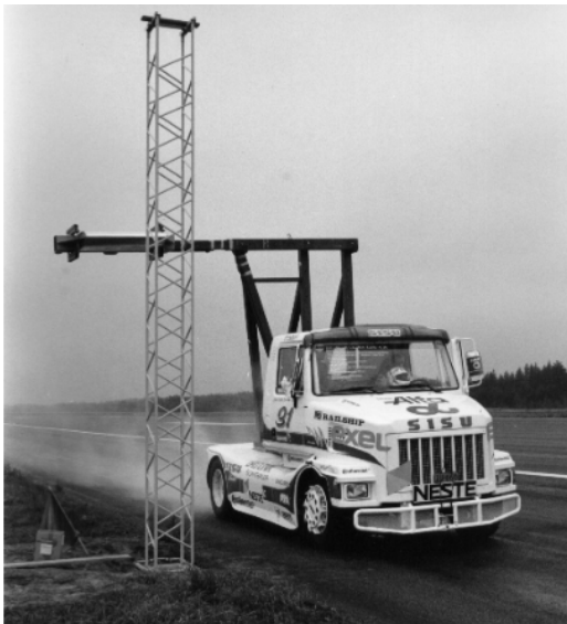
(a) Elevated impactor.[13]
