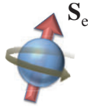
Figure 1.1: The quasi-classical picture of a free-electron spin arising from the rigid spherical electron with total charge -e spinning around its own axis. The intrinsic spin is \mathbf{S}_e with magnitude |\mathbf{S}_e| = \hbar/2 . Although modern physics views the electron as a “point-like” particle, the classical picture is still popular and widely used due to its intuitive form.
