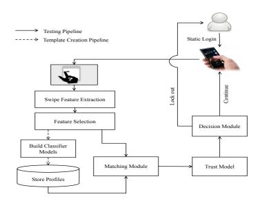
Figure 9.1: Block diagram of the proposed CA system for mobile devices.
