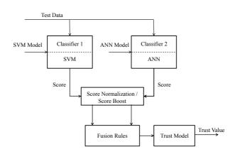
Figure 6.5: Block diagram of the *Trust Calculation* module (see Figure 6.3) with score normalization and/or score boosting.
