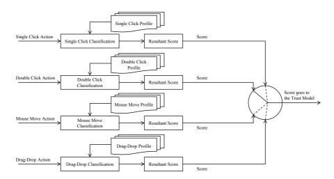
Figure 8.9: Block diagram of the Mouse Matching Module.
