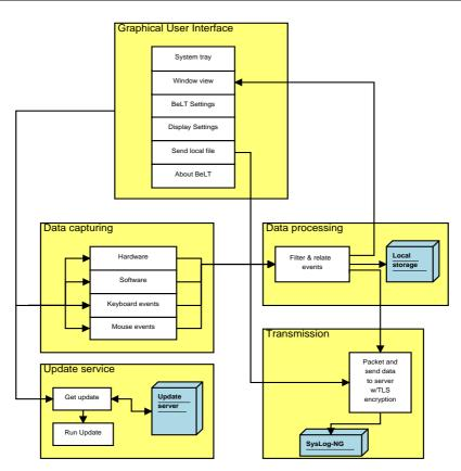
Figure A.2: Logical view of the BeLT client application.
