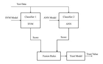
Figure 6.4: Block diagram of the *Trust Calculation* module (see Figure 6.3) without score normalization or score boosting.
