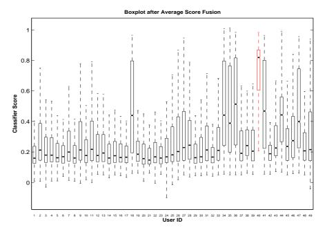
Figure 6.6: Distribution of the classifier score after average fusion for the best performing user for VP-2. Red mark of this box-plot is the genuine user's score distribution.
