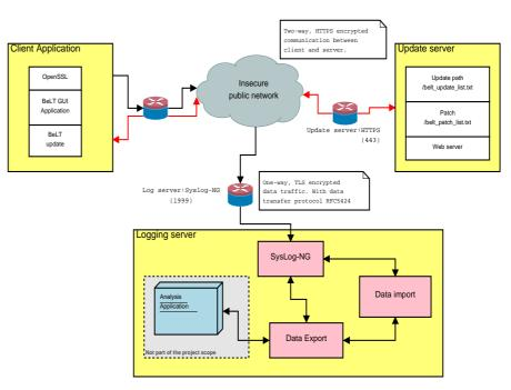
Figure A.1: Deployment diagram of BeLT system.
