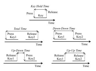
Figure 5.3: Keystroke Dynamics Features
