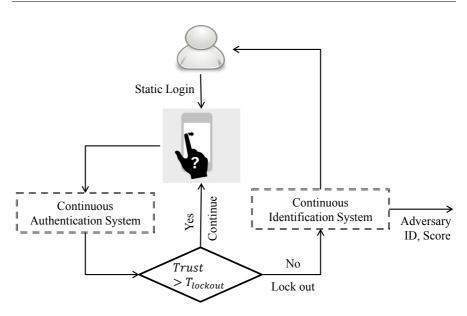
Figure 10.1: Block diagram representation of the architecture of our system.
