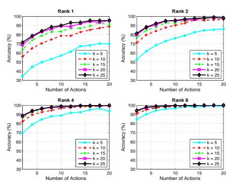
Figure 12.5: Results obtained from S2 for different k value.
