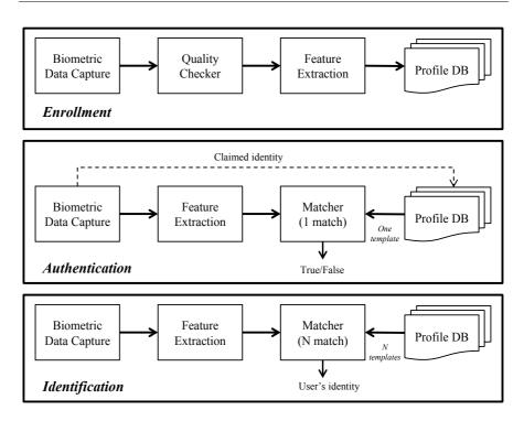
Figure 2.1: Block diagram of a biometric system [65].
