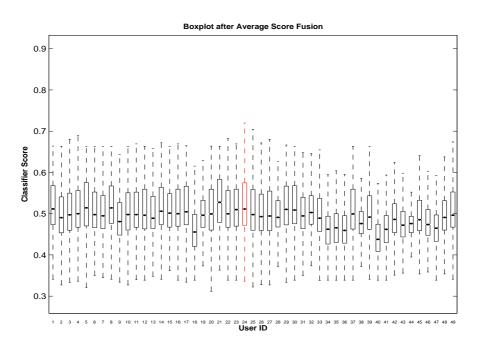
Figure 6.7: Distribution of the classifier score after average fusion for the below average performing user for *VP*-2. Red mark of this box-plot is the genuine user's score distribution.
