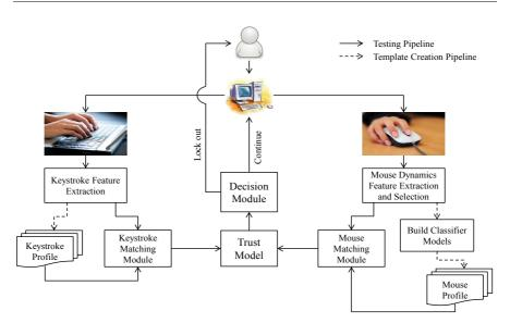
Figure 8.7: Block diagram of the proposed system.
