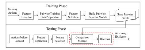
Figure 10.2: Block diagram representation of our Continuous Identification System.
