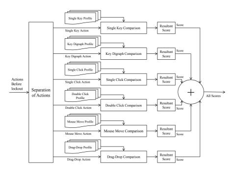
Figure 11.1: Expanded block diagram of the CIS Comparison Module.
