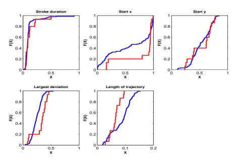
Figure 12.2: Cumulative Distribution of selected features for  $CIS_1^8$  of *Dataset-3*. The blue CDF are generated from the data of user 8 and the red CDF are generated from the data of the user 1.
