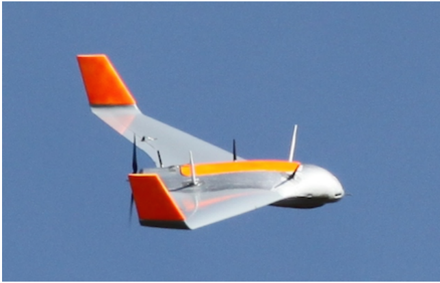
Figure 1. X-8 UAV from Skywalker Technology Co, Ltd.
