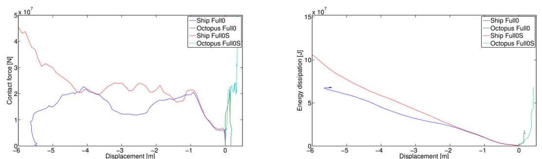
It is seen that there is an apparent difference in both the force deformation curves and in the Energy dissipation- deformation curves. Focusing on the ship, where there is the most damage and energy absorption, it is seen that the simplified analysis over predicts the strength of the bow.
