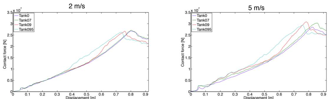
It is seen that the contact force is higher for a given displacement for the cases with ballast water. The analyses with filling levels of 90 % and 95% reach their maximum load at a smaller displacement. They fail earlier because the increased pressure inside the ballast tank changes the stiffeners buckling shape. The maximum load is however in the same range or slightly lower than the maximum load of the empty tank.
