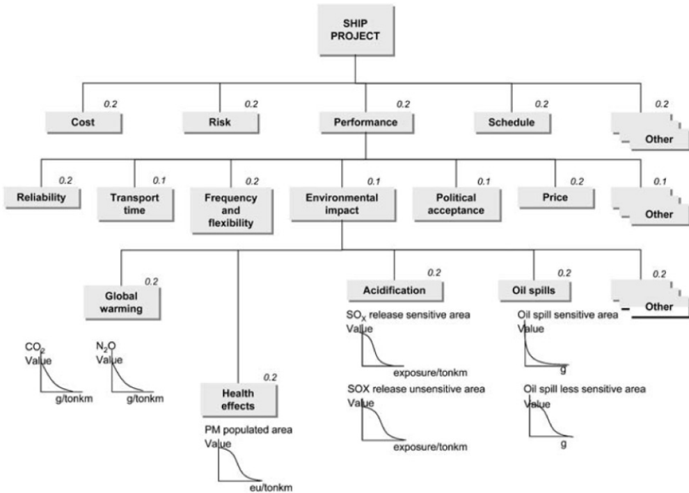
Figure 16: Scoring functions in ship design for the evaluation of environmental impact [117]
