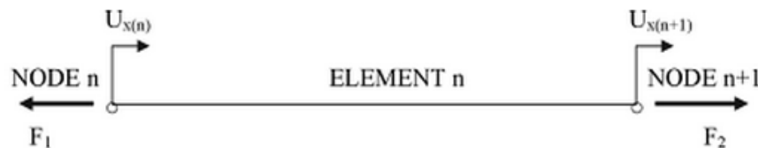
Figure 12 A one-dimensional model (2-nodes and one element) represent its displacement ( U_{x(n)} & U_{x(n+1)} ) in x-direction (Steffen, 2012)
