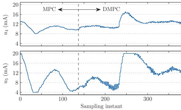
Figure 3: C.S.T.H. experiment — controller performance: manipulated inputs.
