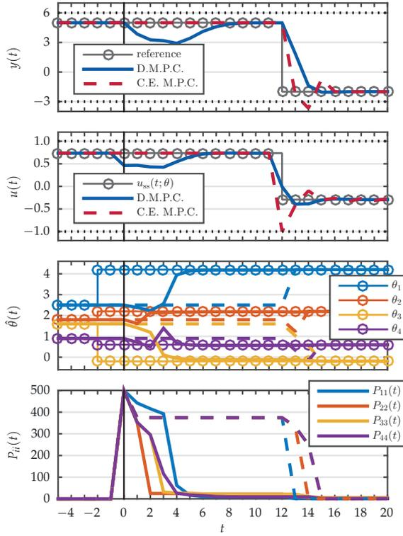
Figure 2: A comparison of certainly-equivalence (C.E.) M.P.C. (dashed, heavy lines) and D.M.P.C. (solid, heavy lines).
