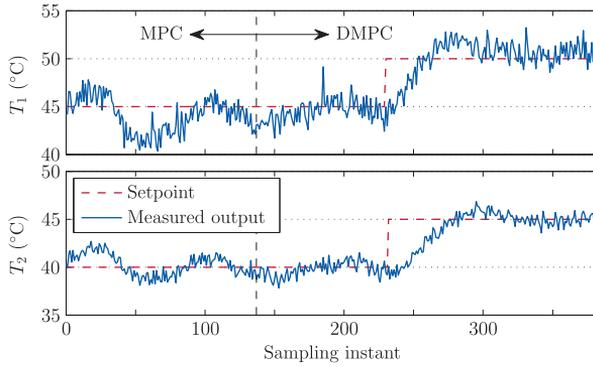
Figure 2: C.S.T.H. experiment — controller performance: setpoint tracking.
