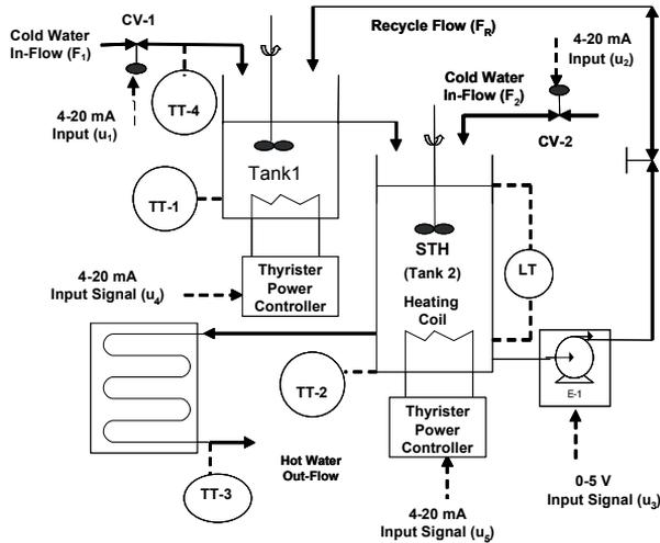
Figure 1: Schematic diagram of the C.S.T.H.
