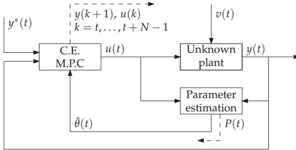
Figure 1: Block diagram illustrating a standard certainty-equivalence M.P.C. structure.
