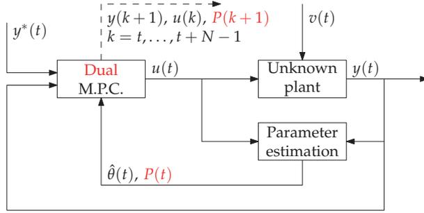
Figure 2: Block diagram illustrating a dual model predictive controller.
