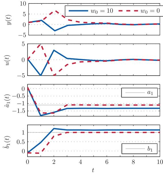
Figure 3: Representative example simulation comparing the variance-minimizing D.M.P.C. defined by (22) with  $w_0 = 10$  and the standard C.E. M.P.C. from Section 2.3 (corresponding to  $w_0 = 0$ ).
