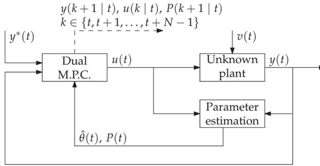
Figure 1: Block diagram illustrating the adaptive D.M.P.C. structure. The dashed line illustrates variables predicted by the D.M.P.C.
