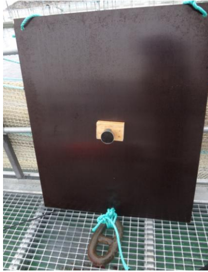
Figure 9: One wooden plate for holding the transducer.
