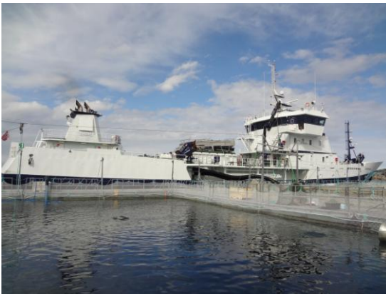
(a) Well boat: fish are transferred from well boat into the plant through a pipe.
