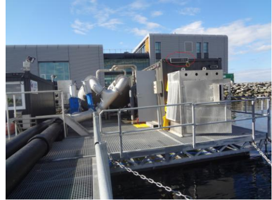
(f) One electronic board displays the number of fish per minute passing through the main pipe.
