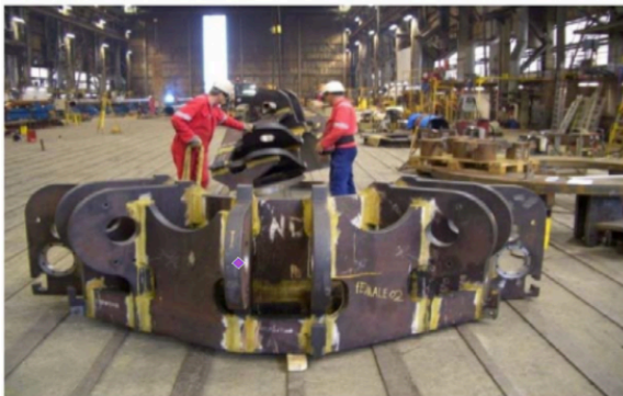
Figure 2.4 - DAT system with tensioner ring [14]
