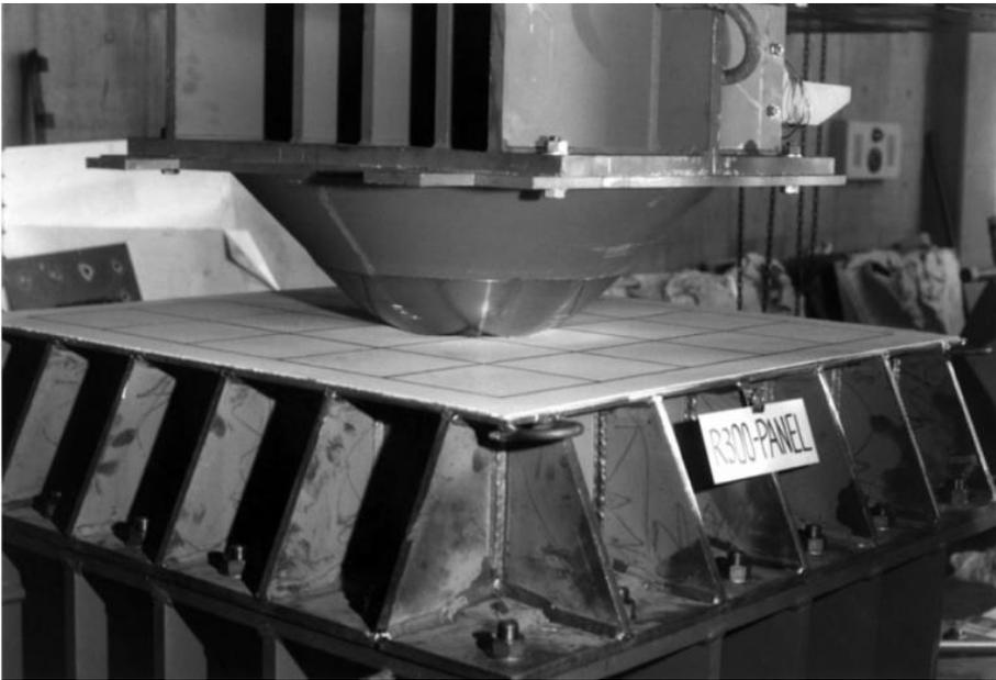
Figure 14 - Quasi-static experimental test setup (49)
