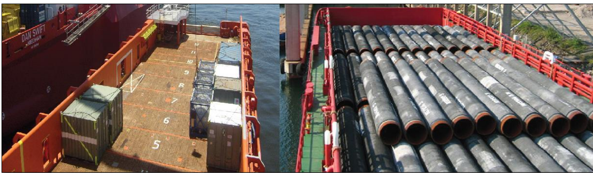
Figure 17 - Storage of containers and pipes on PSV deck, Skandi Waveney and Skandi Rona. Figures taken from www.dof.no (11.04.2013)
