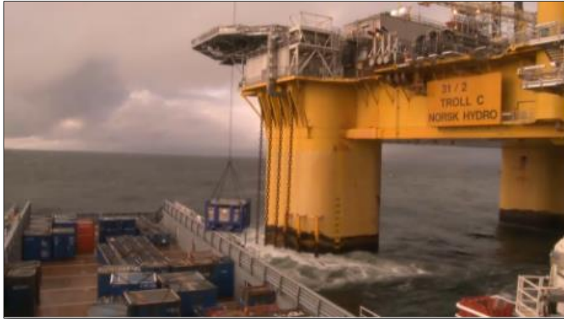
Figure 15 - Offloading operations from a PSV to Troll C. Figure taken (08.04.2013) from http://www.logistikkportalen.no
