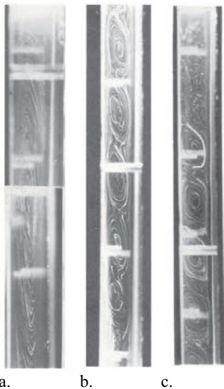
Figure I-1. Streak photographs from Seki et al. (1978), A = 15 , a) Ra=1.33 \cdot 10^5 , b) Ra=2.9 \cdot 10^5 , c) Ra=1.4 \cdot 10^8 .
