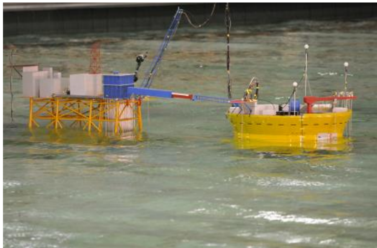
Figure 2: Model test of the FSU at the Marintek basin (Muthanna, 2011)
