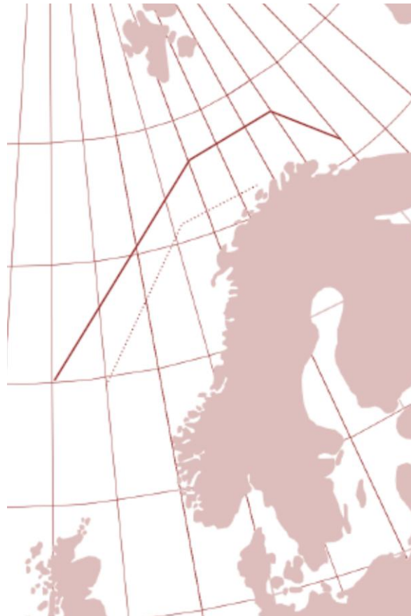
FIGURE 77 - LIMITS OF SEA ICE IN THE BARENTS SEA WITH ANNUAL PROBABILITY OF EXCEEDANCE OF 10^{-2} (SOLID LINE) AND 10^{-4} (DOTTED LINE). FROM NORSOK N-003
