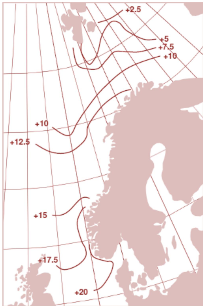
FIGURE 73 - HIGHEST SURFACE TEMPERATURE IN THE SEA WITH AN ANNUAL PROBABILITY OF EXCEEDENCE 10^{-2} (THE TEMPERATURES ARE GIVEN IN °C) [116]
