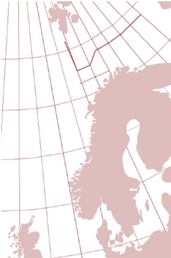
FIGURE 78 - LIMITS FOR COLLISION WITH ICEBERGS WITH A PROBABILITY OF EXCEEDANCE OF 10-2 (SOLID LINE) AND 10-4 (DOTTED LINE). FROM NORSOK N-003
