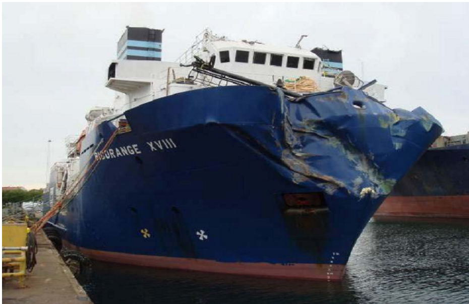
Figure 2.4: The bow of the Big Orange XVIII after collision.
