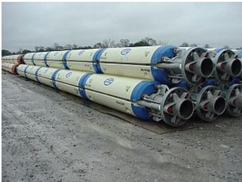
Figure 2.2: Drilling riser joint with buoyancy modules
