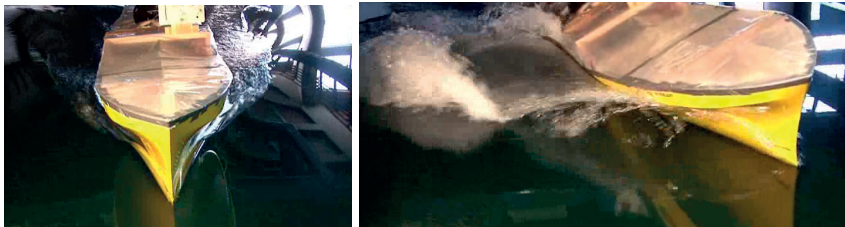
Figure 1.4: Illustrations of non-linear flow around a semi-displacement vessel, Left: Fn = 0.5 , Right: Fn = 0.6 with 10^\circ drift angle, pictures from experiments at INSEAN by Fabbri et al. (2009).
