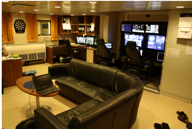
Figure 8.2: Work place and control room onboard KL Saltfjord. The ROV is typically operated by two pilots. Video feeds from the ROV and other information are shown on the monitors.
