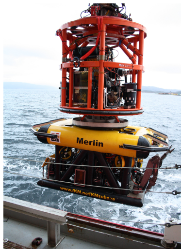
Figure 8.4: ROV attached to TMS while being deployed from the starboard side of ship at the docks of Mongstad.
