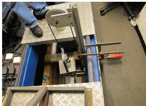
Fig.A.3 Setup for Load Case 3 – Moment about Z-axis
