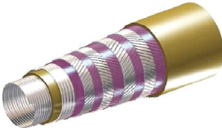
Figure 2.3: Unbonded cross section with four tensile armour wires [3].
