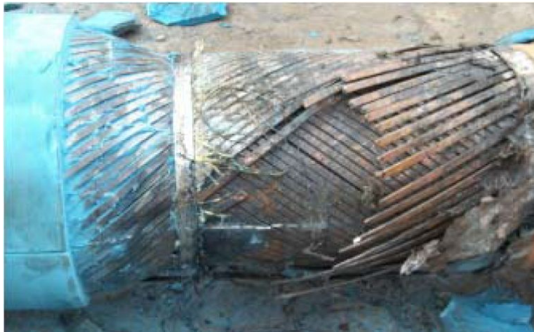
Figure 2.4: Rupture of the tensile armour wires of a flexible pipe [6].
