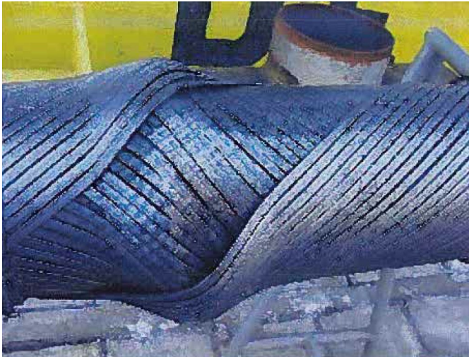
Figure 2.5: Example of bird caging of tensile armour wires [8].
